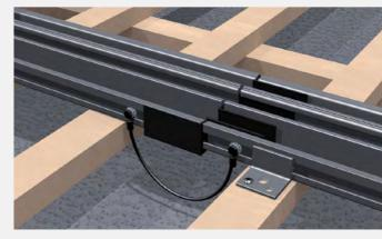
Earthing of IP rail joints of the in-roof system The base profiles of the TRI-ROOF+ in-roof system are securely connected at each joint connection with the TS earthing set 2 at each joint connection. This ensures a connection between the IP rail strands and ensures both effective earthing and increased protection.
