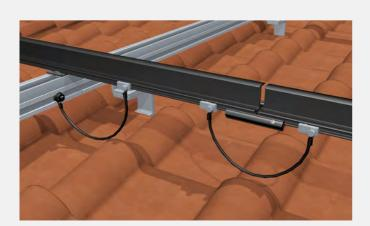
**Earthing of TS rail joints and vertical profiles** The TS earthing set 1 is used to connect all rail joints of the TS insertion profiles to ensure reliable earthing. In addition, TS earthing set 3 is used to create a secure connection between the TS rail sections and the vertical profiles.
