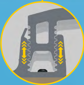
Height-adjustable base plate
