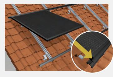
4. Inserting the modules into the TS insertion profiles The modules are inserted into the insertion profiles and are held in place by their own weight - there is no need for additional fastening.
