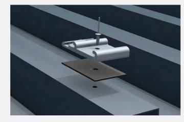
**2. Riveting the SafeClick onto the trapezoidal sheet** The proven SafeClick is mounted directly onto the trapezoidal sheet metal by rivet<sup>1</sup>, whereby considerably fewer fastening points become necessary.
