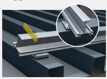
3. Clicking the TS insert profiles into the SafeClick The insertion profiles are clicked into the SafeClick and are floatingly connected to the roof. Damage to the roof and module caused by thermal expansion is thus avoided.
