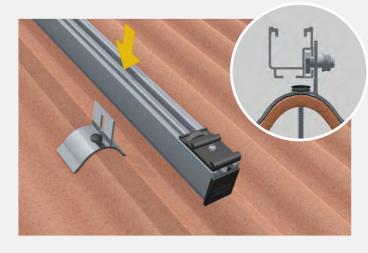
2. Mounting the base profile (UP-X) The pre-assembled profiles are then securely installed on the TS-COR with the M10 hammerhead screw.
